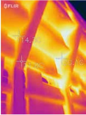
Figure 7.0 - Rear of block A showing the heated party wall from the coils is warmer than the unheated wall
