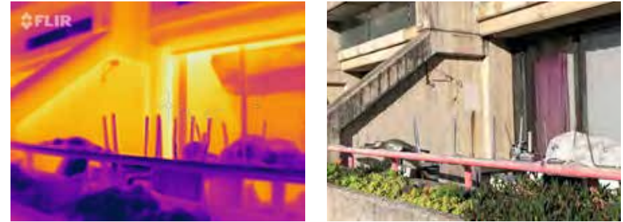
Figure 7 : Front of block A illustrating heat loss and the thermal bridge from the heated party wall. Temperature where the concrete fin meets the window wall shows 15°C. The thermal image was taken at 8pm to prevent the heat from the sun affecting the image. The photograph was taken the following day.
