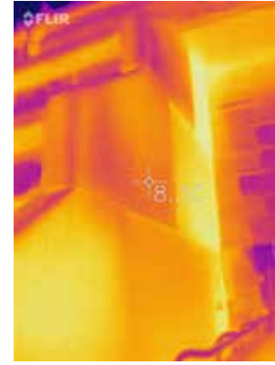
Figure 7.2 - Eastern end wall of block A illustrating heat loss from the heating coils in the dwellings.
