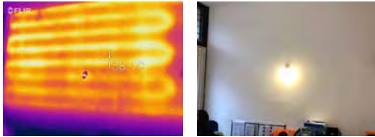
Figure 13: Internal image of a void A3 unit (Mulalley's site office), showing the coil heated party wall in the double height space.
