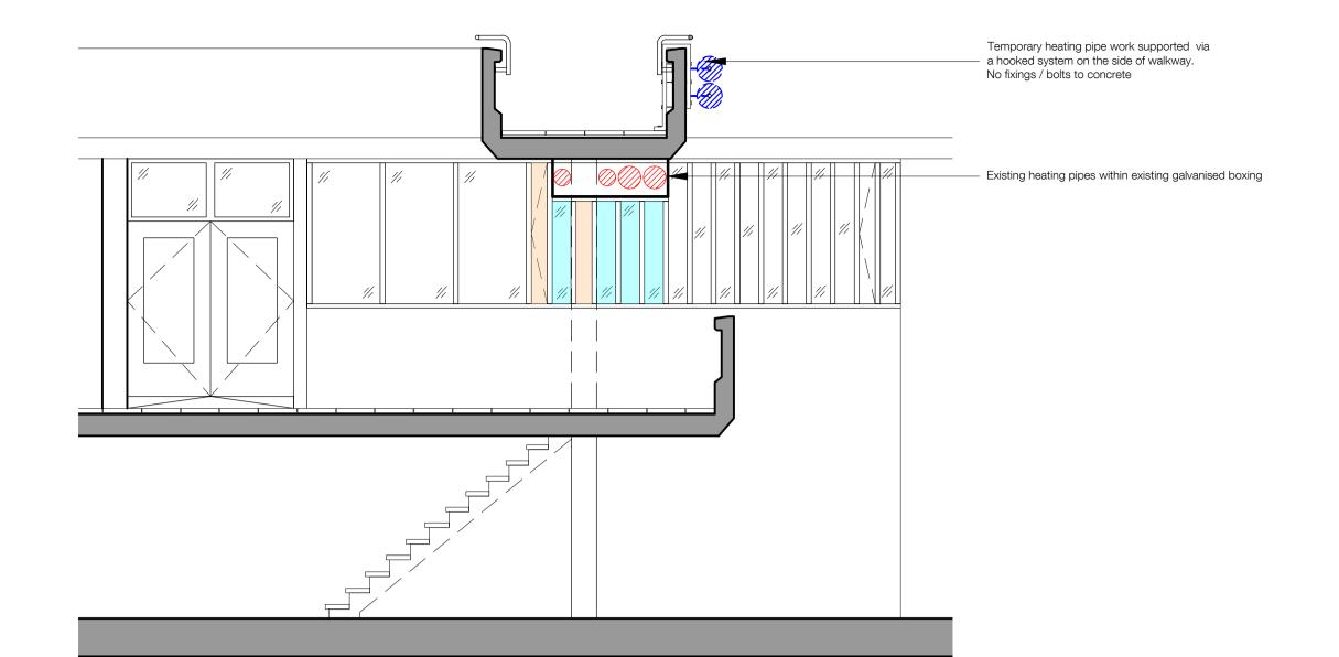
Block A - Section A Through Link Bridge looking towards Housing Office 140005 Existing and Temporary Condition
