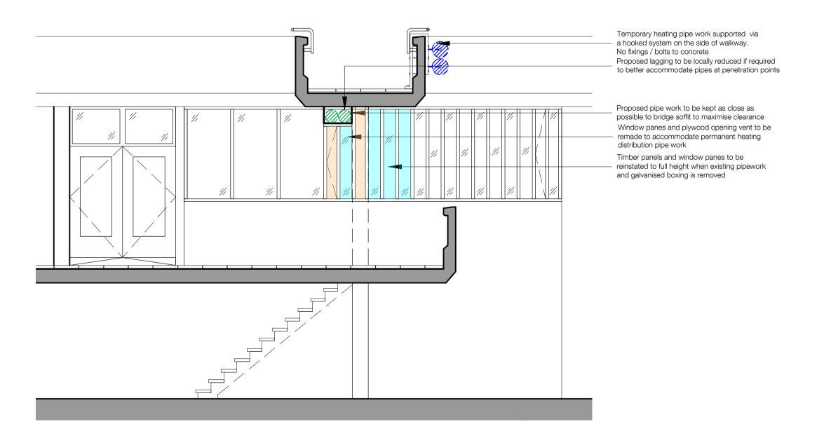
Block A - Section B Through Link Bridge looking towards Housing Office 140005 Proposed Final and Temporary Condition
