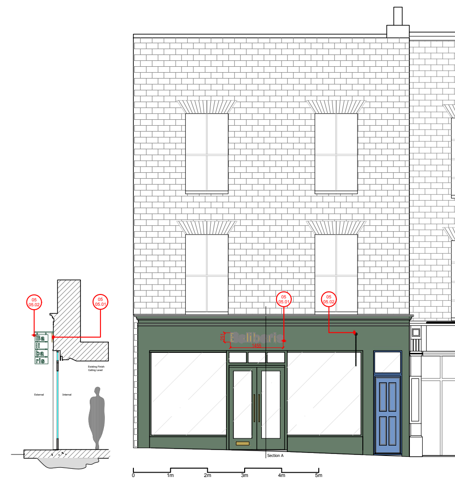
PROPOSED SHOPFRONT ELEVATION & SECTION
