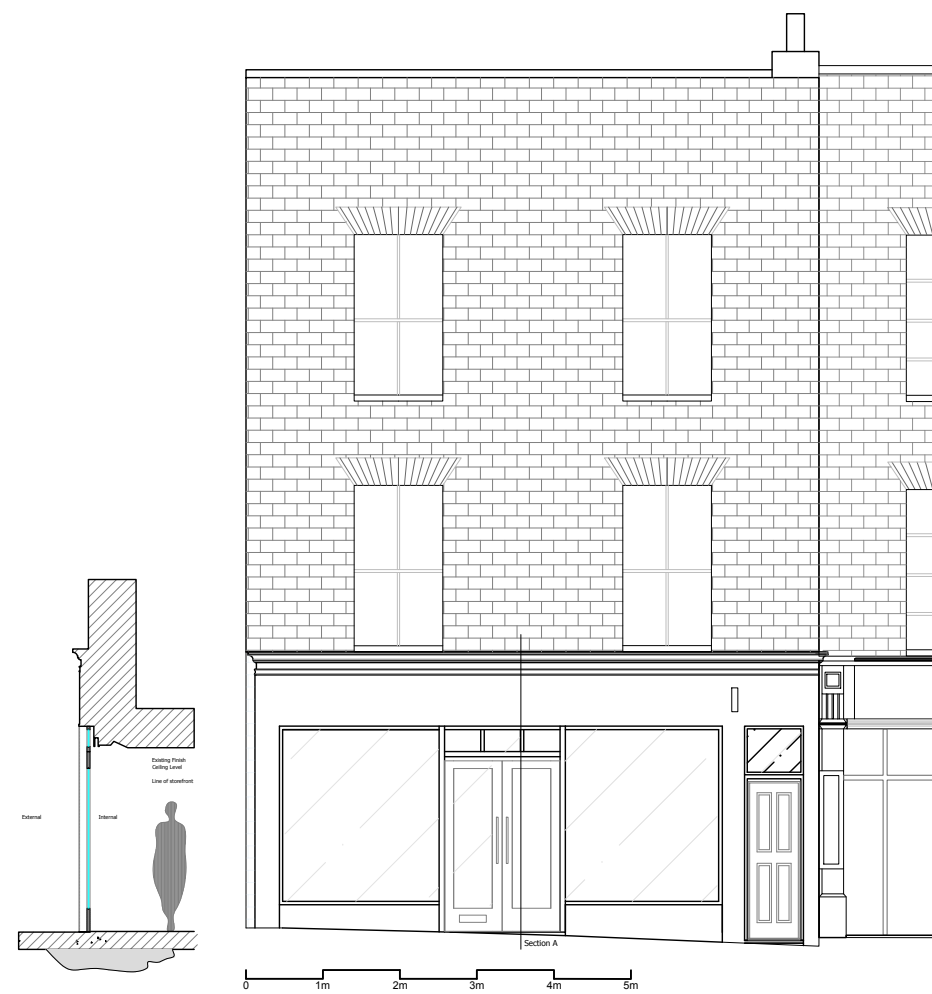
EXISTING SHOPFRONT ELEVATION & SECTION
