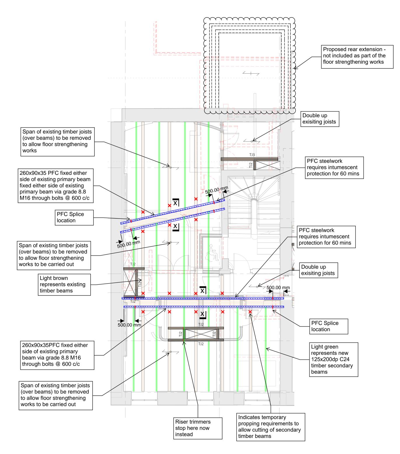
Typical Floor Strengthening Requirements -First and Second Floor Structure (i.e. Ground Floor Ceiling and First Floor Ceiling)
