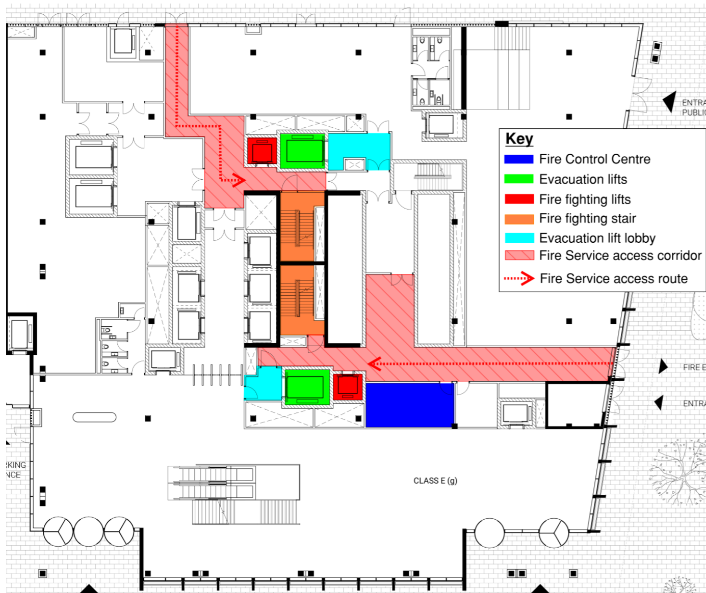
Figure 5 - Firefighting facilities provided within the building. Ground Floor access presented.
