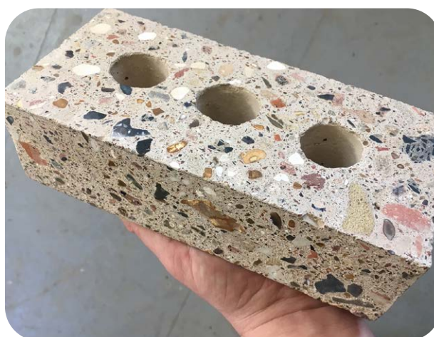
Figure 4.28 Process for manufacturing waste-based bricks from inert materials (above) and reference images of upcycled brick products (below)
