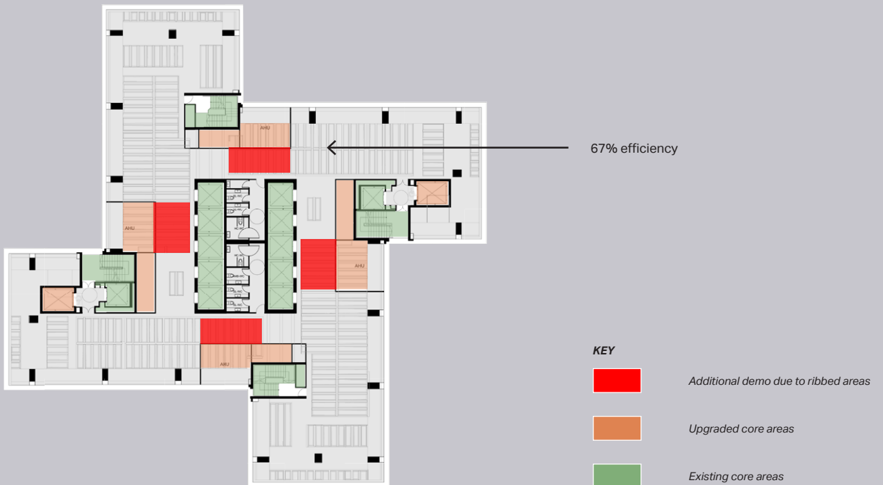
Figure 2.3 Diagram showing erosion of floor slab and exaggerated penetrations due to upgrades to meet current Building Regulations
