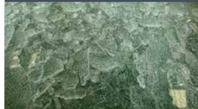
Class A – clean clear glass cullet with no contamination which can be used back in the float line by re-melting.
