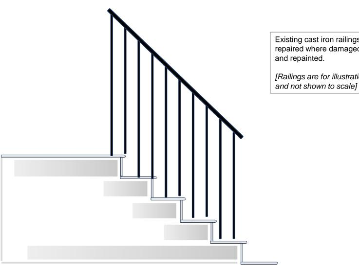
Existing cast iron railings retained and repaired where damaged. Stripped
