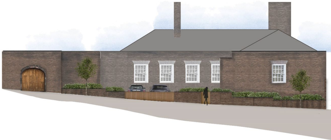
Figure 3a – Proposed Front (North-West) Elevation showing new low-level wall and gate. The design mirrors the form of the existing building which follows the slope of the terrain. We propose using narrow red brick to build the wall, to match the original building, and solid wood for the gate.
