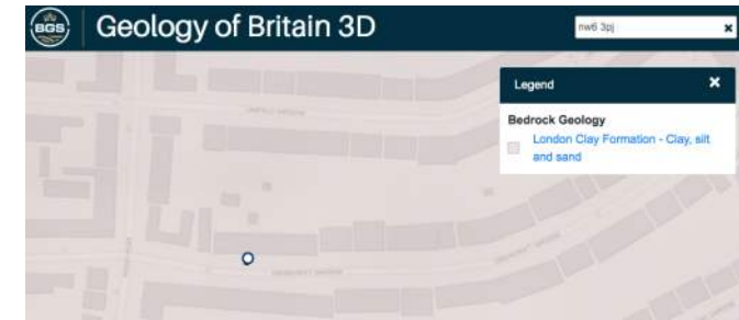
Figure 03:- The Geological Map for the Property (shown circled) indicates London Clay Formation - Clay, silt and sand.
