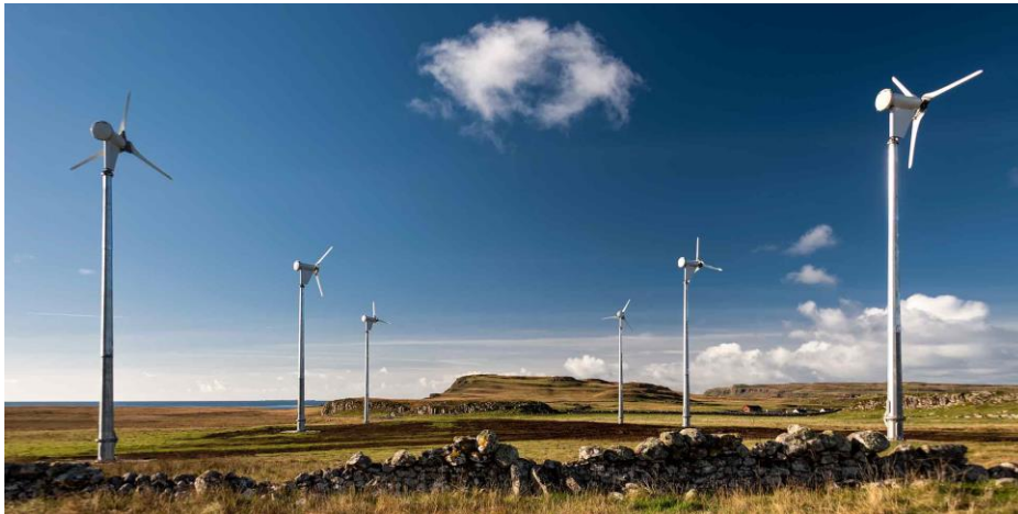
Figure 9: Typical Small Scale 6kW Wind Turbine
