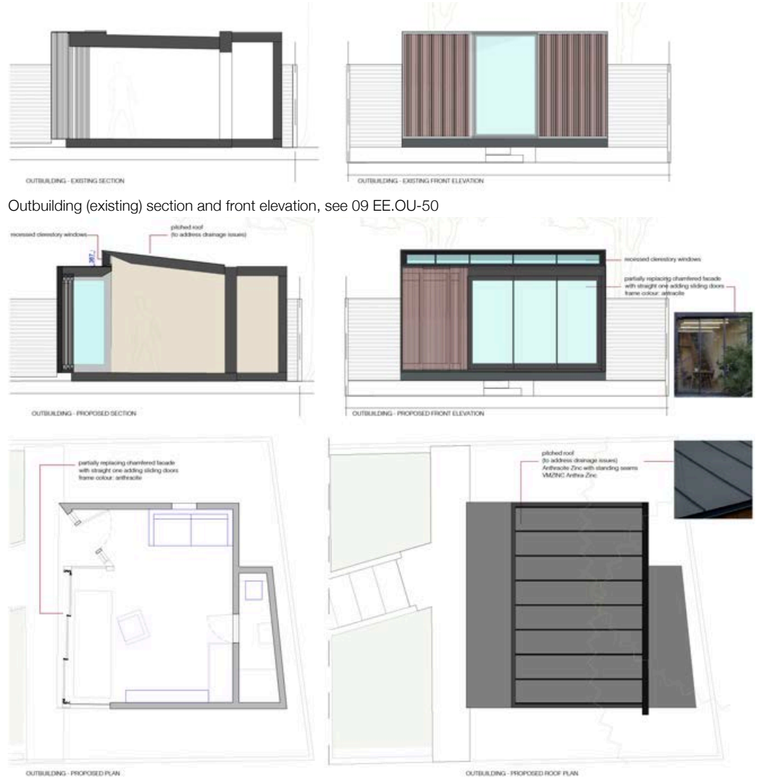
Outbuilding (proposed) section and front elevation; plan and roof plan. See 10 PP.OU-50
