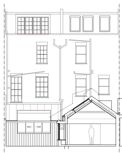
Image above: 1:200 scale section through proposed extension.
