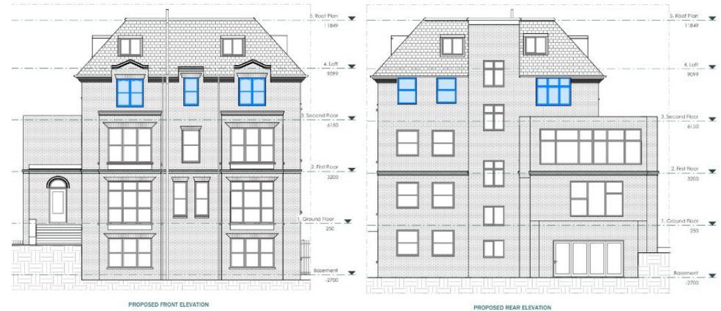
Fig 5: Proposed front elevation (left) and proposed rear elevation (right)
