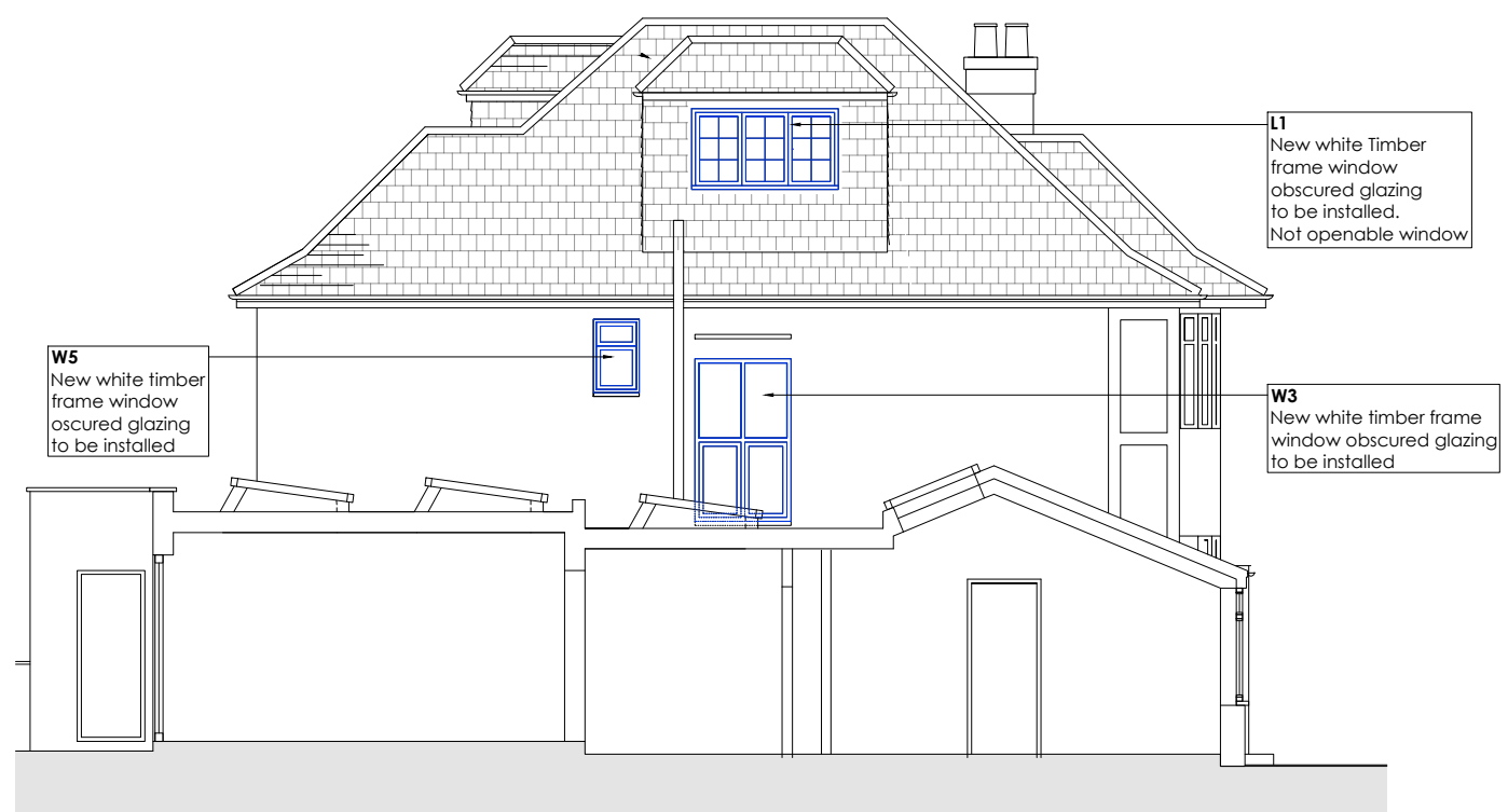
1 AS PROPOSED NORTH SIDE ELEVATION SCALE 1:100@A3
