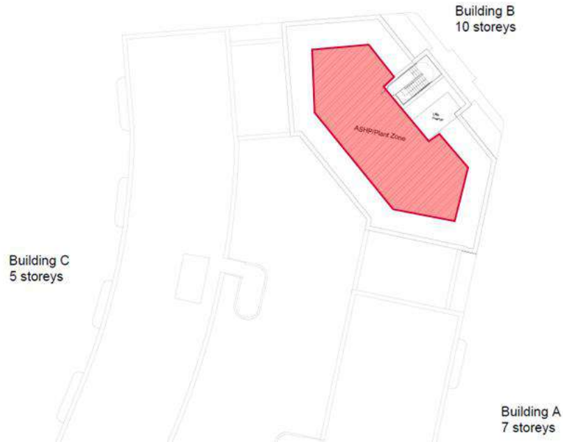
Figure 4.7 Proposed roof-level plant space allocation
