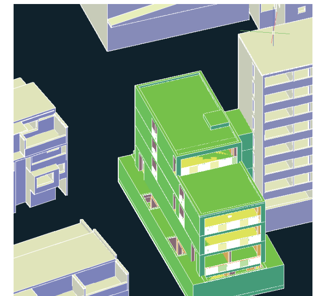
FIG 3 _ Modelling diagram showing no impact on neighbouring windows
