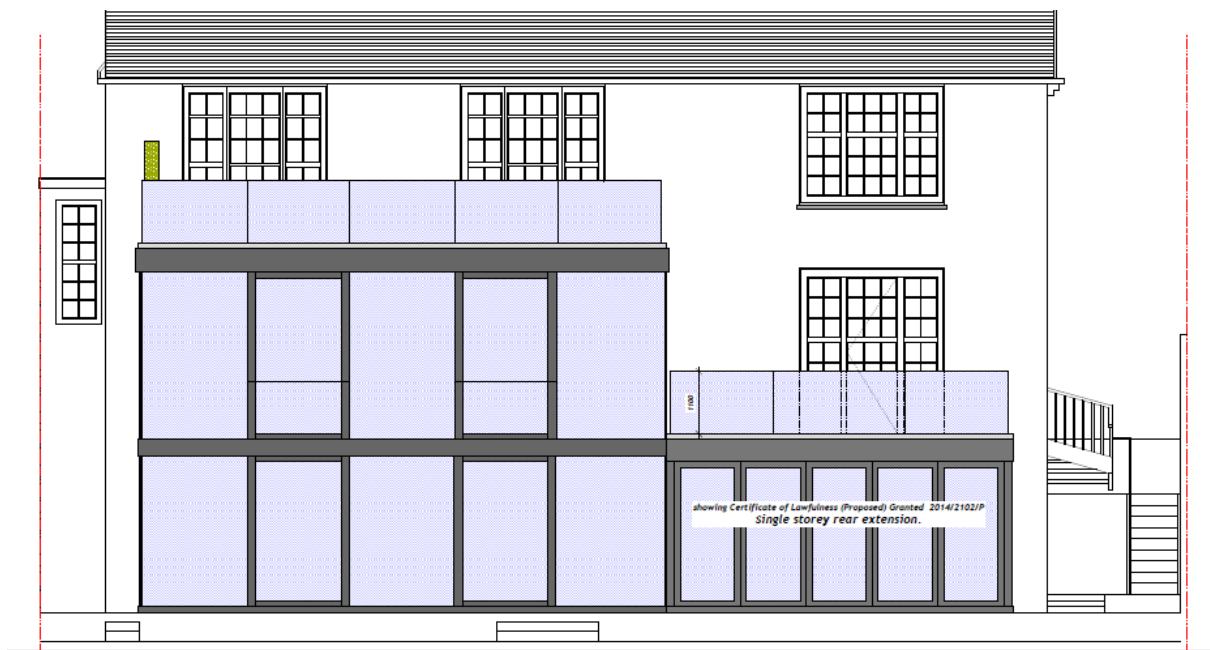
Figure 6 (above): Drawing of the proposed scheme, which differs from Figure 5 in that it features a glass balustrade and the window behind the balustrade has been replaced by a door.
