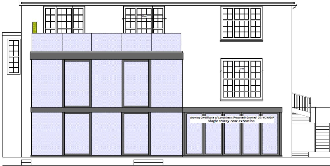
Figure 5 (above): Drawing of the rear elevation as existing and also including the (as yet unbuilt) single storey rear elevation that does not require planning permission and was confirmed as permitted development as part of lawful development certificate application ref. 2014/2102/P.
