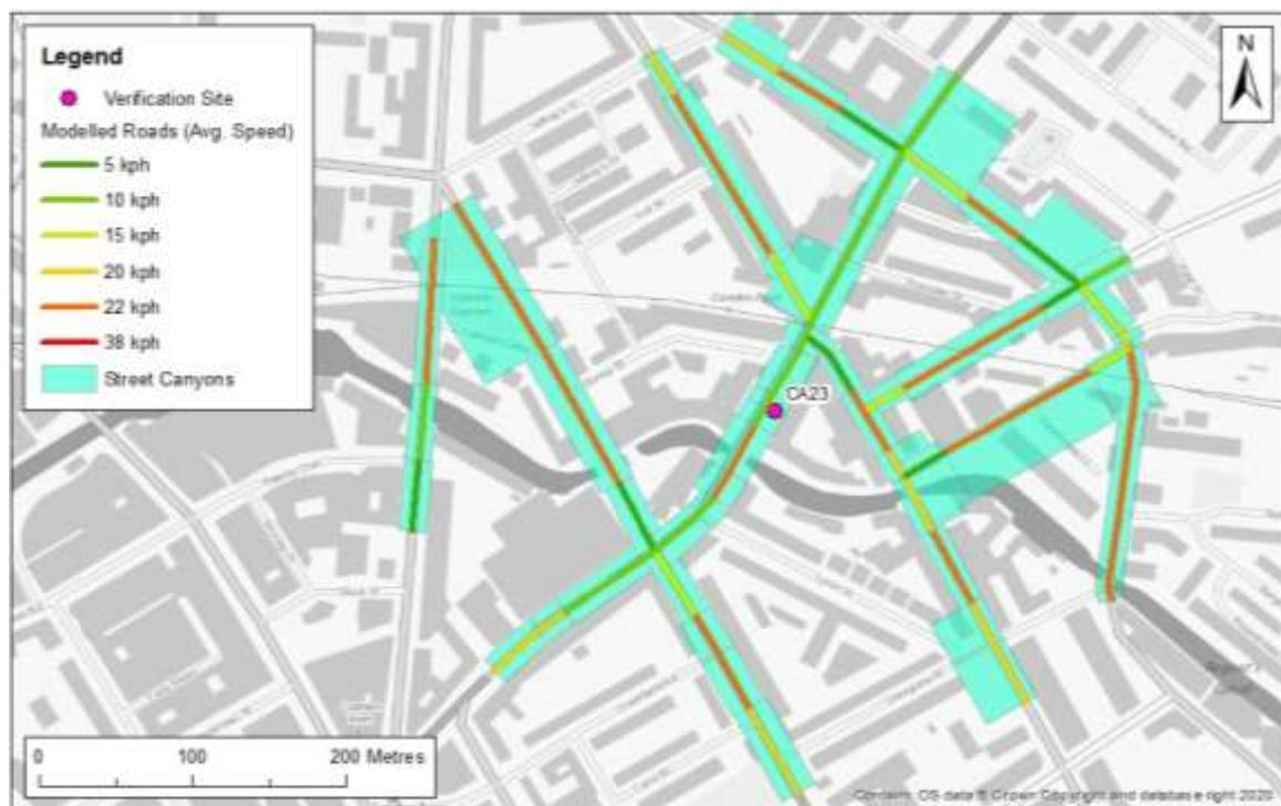
**Figure E.2: Modelled Road Network (inc. Avg. Speeds (kph) and Modelled Street Canyons); Verification Area**
