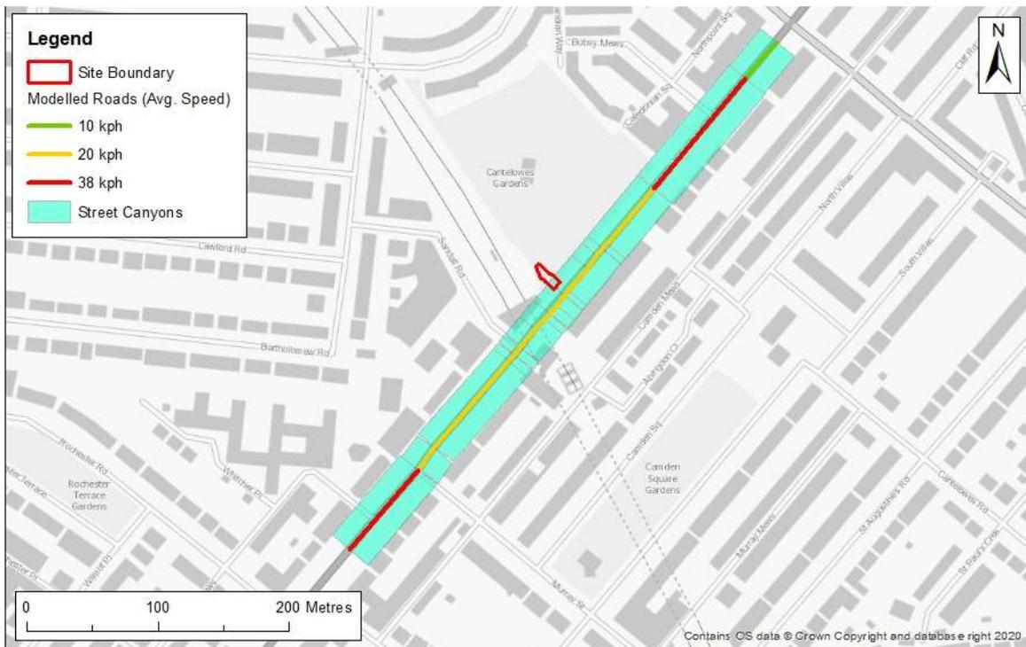
**Figure E.1: Modelled Road Network (inc. Avg. Speeds (kph) and Modelled Street Canyons); Site Area**
