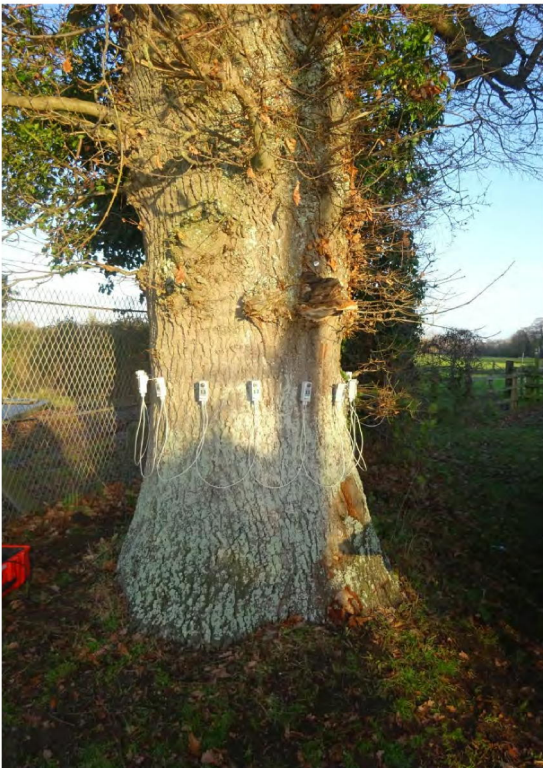
Mature Oak tree with Arbotom sensors around the stem
