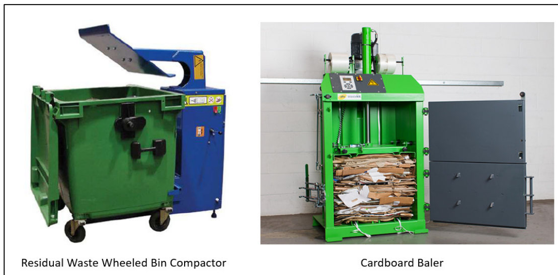
Figure 3.1: Residual Waste Compactor and Cardboard Baler
