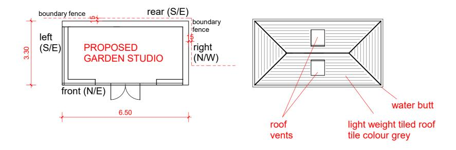
PROPOSED GARDEN STUDIO (for private use as a garden room for the homeowner) the outbuilding is ancillary to the main dwelling width 3.3m, length 6.5m, max hgt 2.9m rear & right side elevation to be facing brick, anthracite grey upvc frames to the front & left side elevation, glazing clear, light weight tiled roof, tile colour grey, 2 x roof vents drainage to water butt, boundary treatments to remain same, existing outbuilding (shed) to be removed
