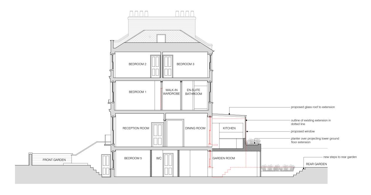
$01 \, \tfrac{\text{PROPOSED SECTION A-A}}{\text{scale 1:100}}$
