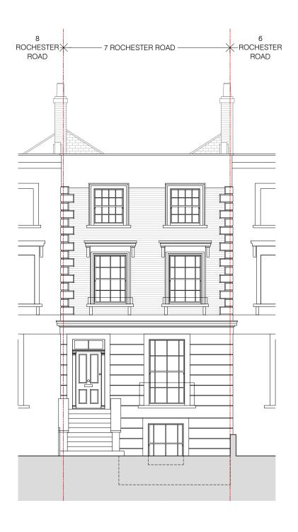
$01 \; \frac{\text{EXISTING FRONT ELEVATION}}{\text{scale 1:100}}$
