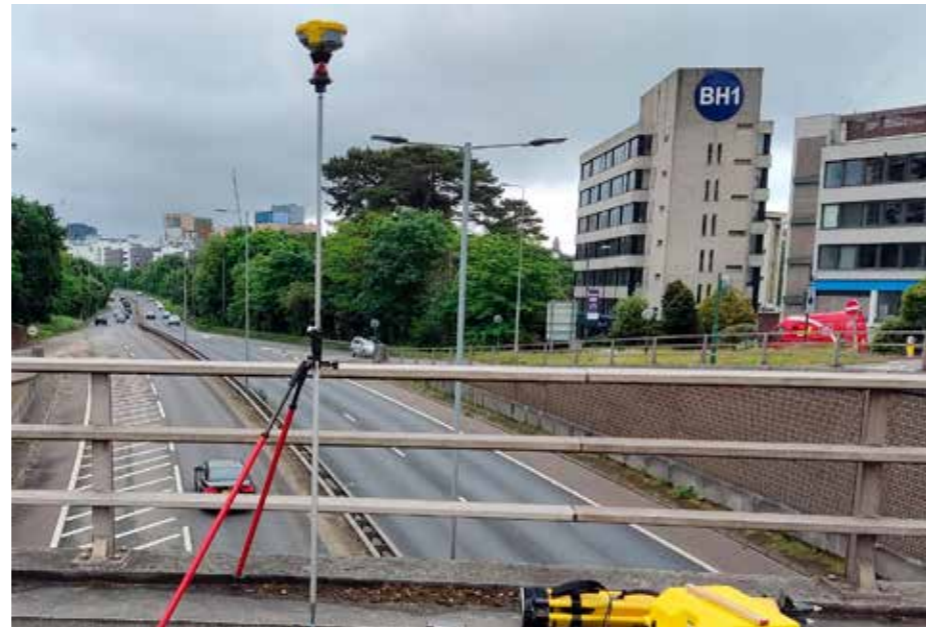
7: Field survey being carried out, GNSS receiver
