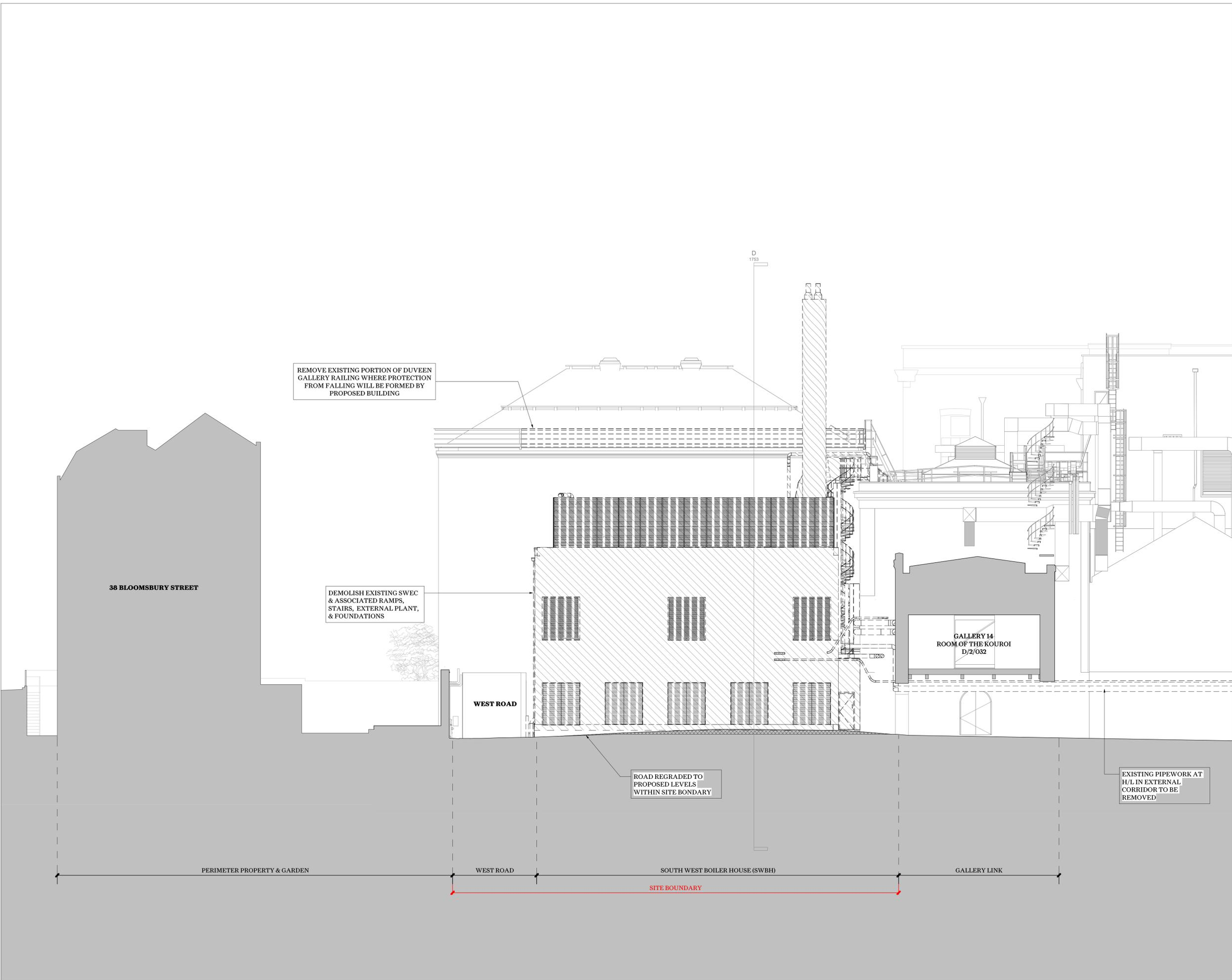
REMOVE EXISTING PORTION OF DUVEEN GALLERY RAILING WHERE PROTECTION FROM FALLING WILL BE FORMED BY PROPOSED BUILDING
