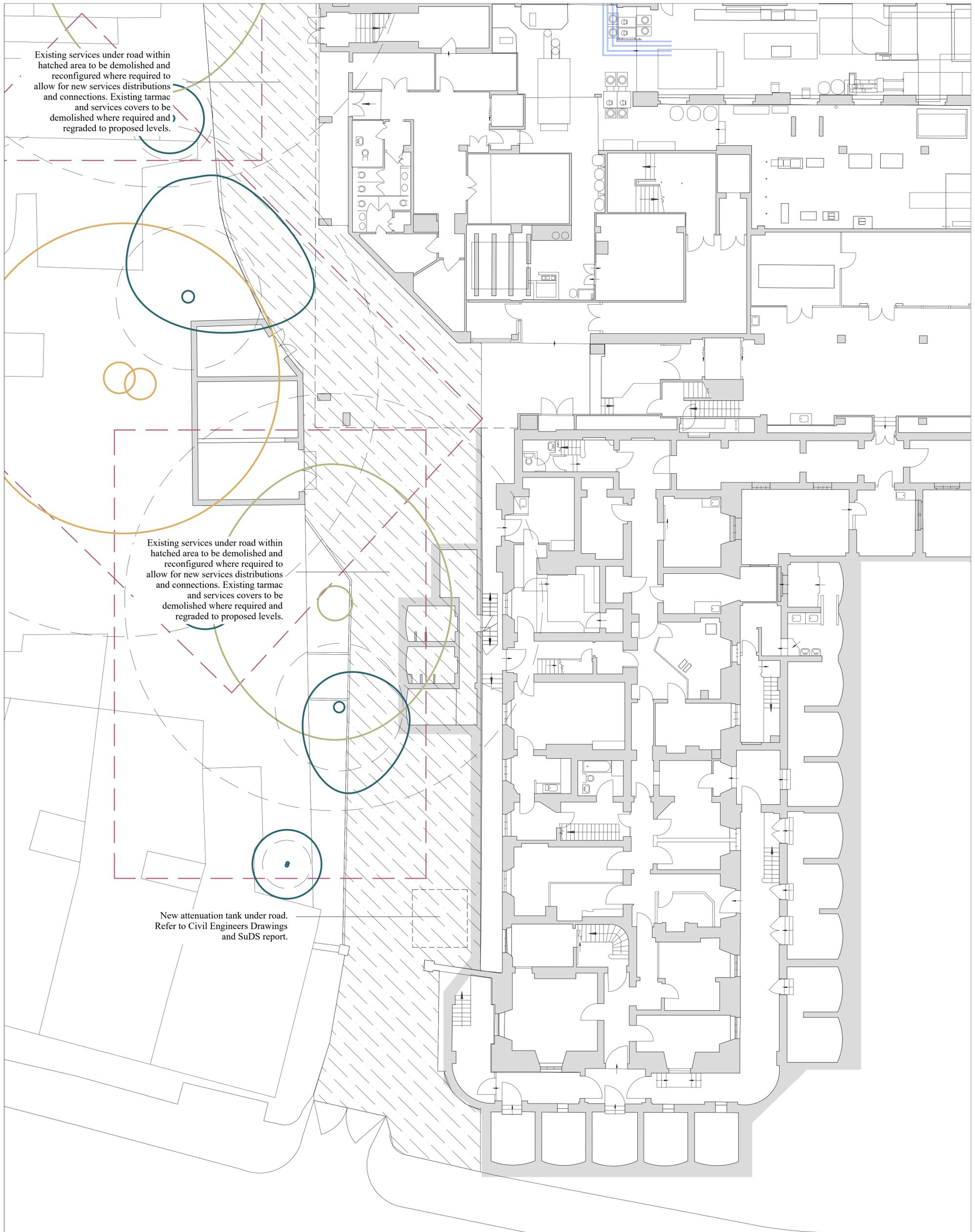
Existing services under road within hatched area to be demolished and reconfigured where required to allow for new services distributions and connections. Existing tarmac and services covers to be demolished where required and regraded to proposed levels.
