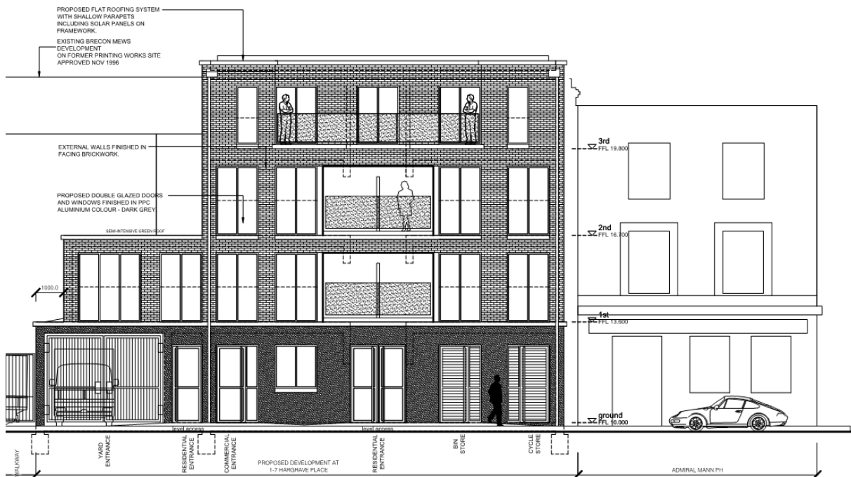
Figure A: The host building as originally approved in relation to the height of the public house next door (to the right)
