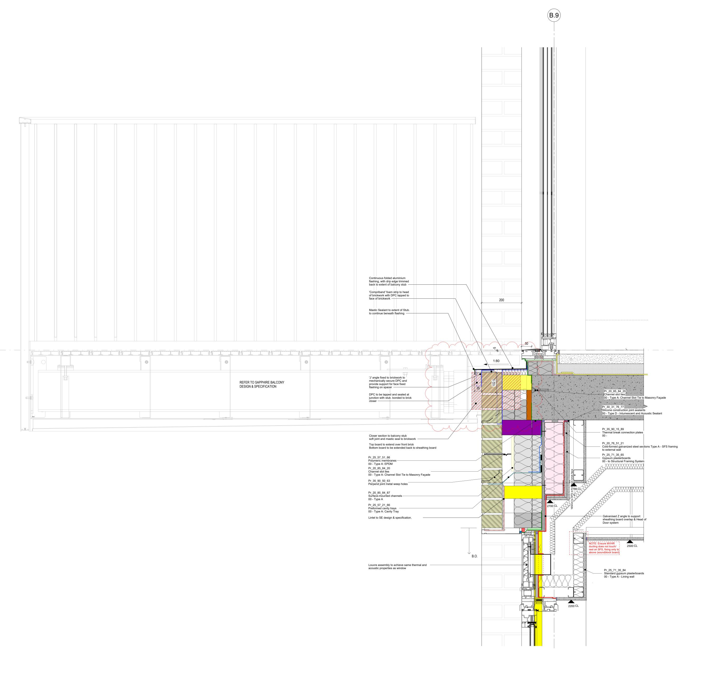
Balcony section detail to EW02A- Typical @ Masonry Support to NVHR + Balcony 1:5
