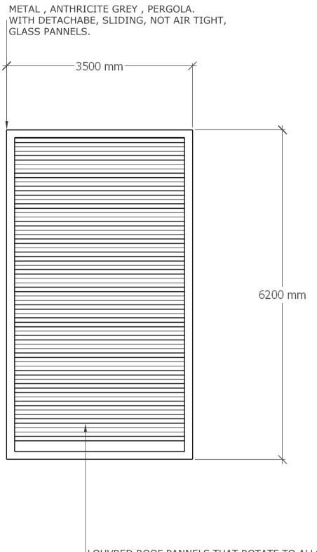
LOUVRED ROOF PANNELS THAT ROTATE TO ALLOW SUNLIGHT AND AIR FLOW DURING GOOD WEATHER. ANTHRICITE GREY IN COLOUR.
