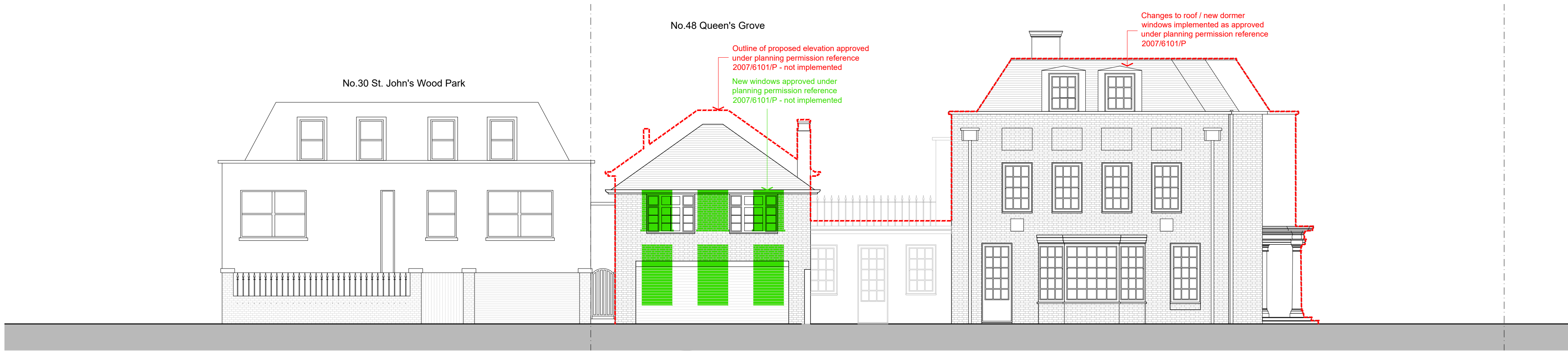
EXISTING FRONT (SW) ELEVATION (SHOWING ADJOINING PROPERTY & EXISTING MAIN HOUSE) Scale 1:100 @ A1
