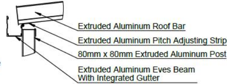
Wall Plate & Roof Bar Section
