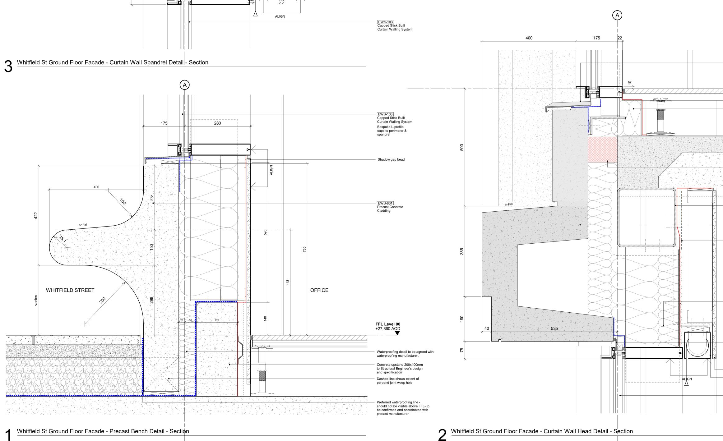
Whitfield St Ground Floor Facade - Precast Bench Detail - Section
