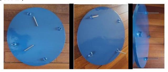
7 cm screws to go into the brick mortar
