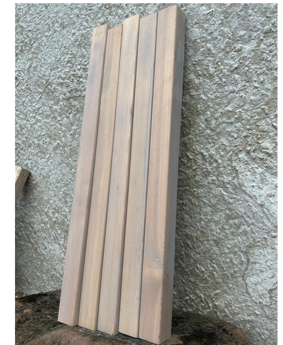
Stained Timber sample, ENVIROGRAF Clear Intumescent coated, slatted and rebated joints. To be used for timber bike and bin enclosure adjacent to gate, and for plant enclosure at the rear of the yard.
