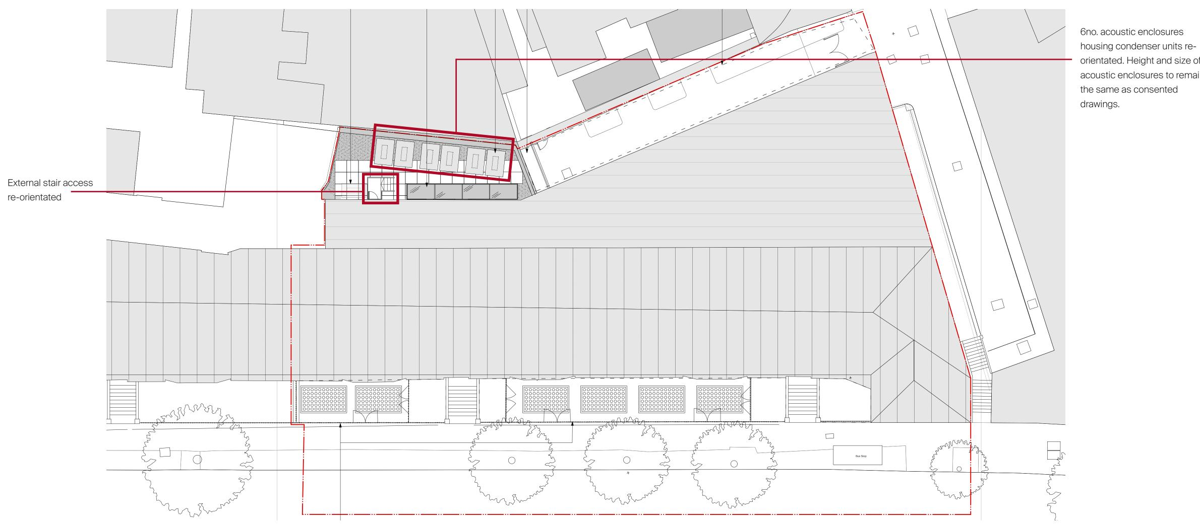
orientated. Height and size of acoustic enclosures to remain the same as consented drawings.
