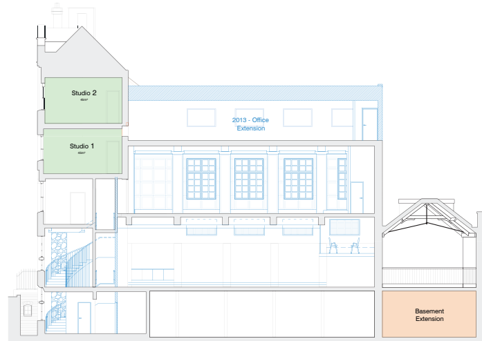
Proposed section showing the single storey office extension, basement extension and residential units at the frontage building
