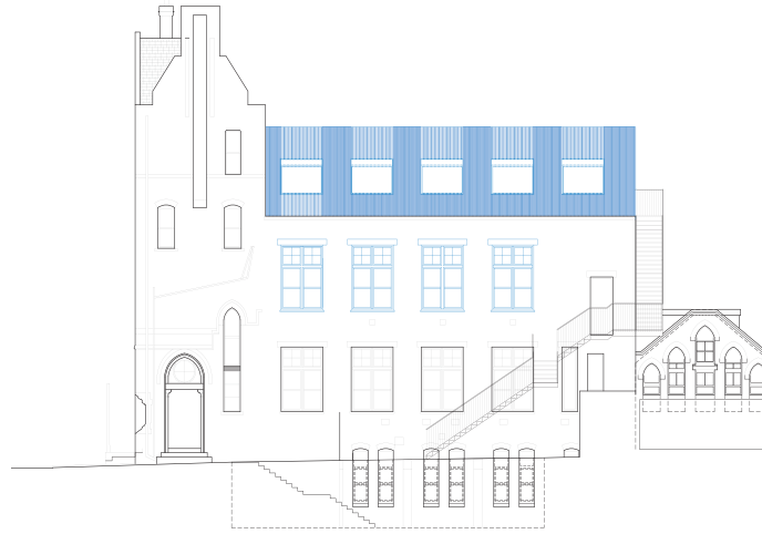
Proposed elevation showing the single storey office extension
