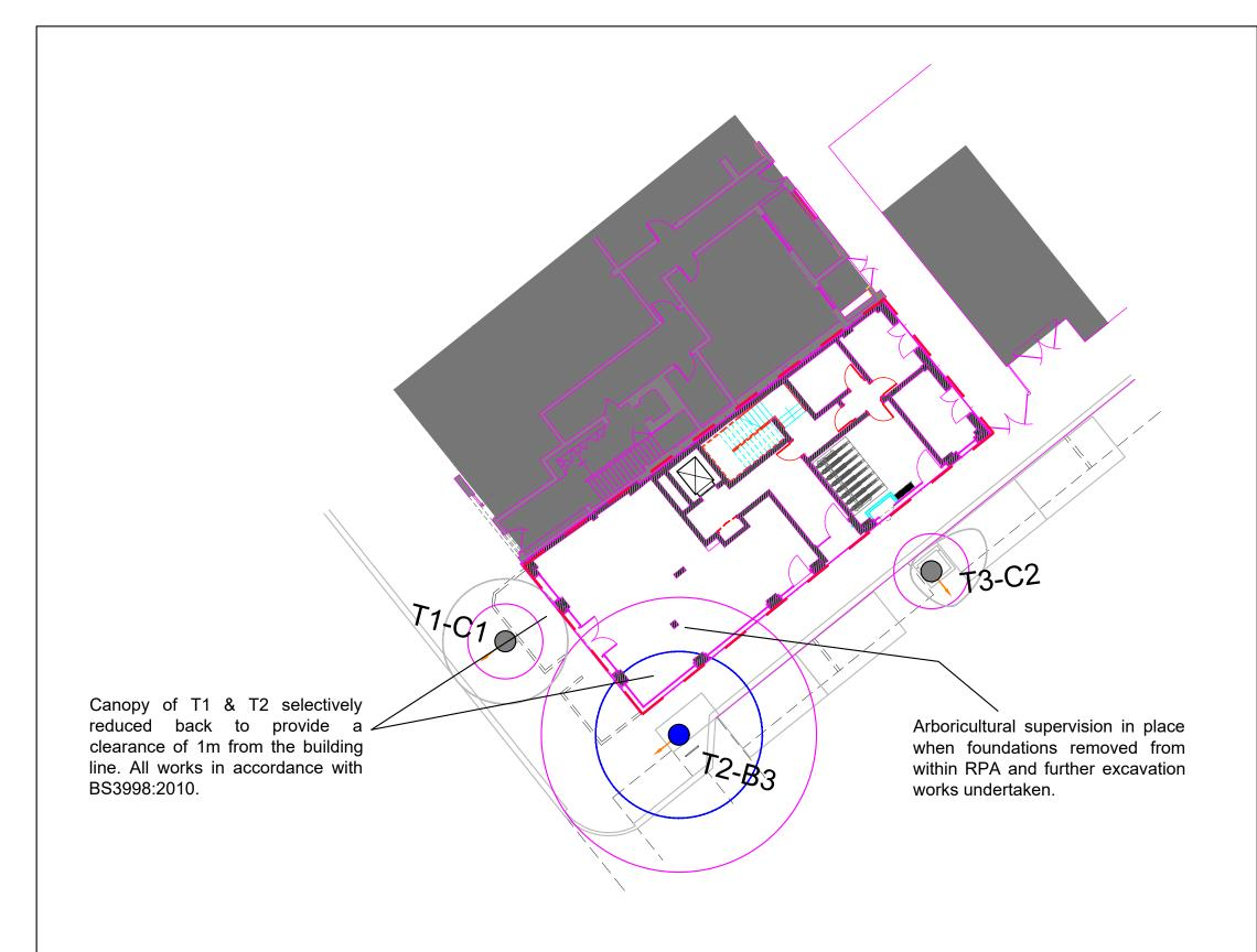
A protective barrier will be set up to prevent collision damage occurring to the trees during works, where permitted on the public highway. Demolition works, deliveries etc will be undertaken in a manner to ensure the trees are suitably protected.
