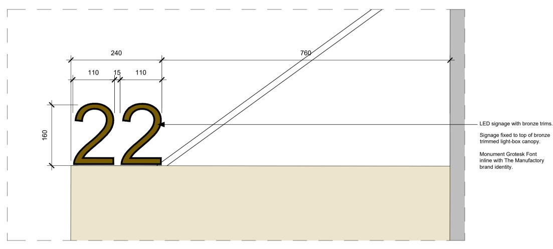
2. Elevation detail Scale: 1:5
