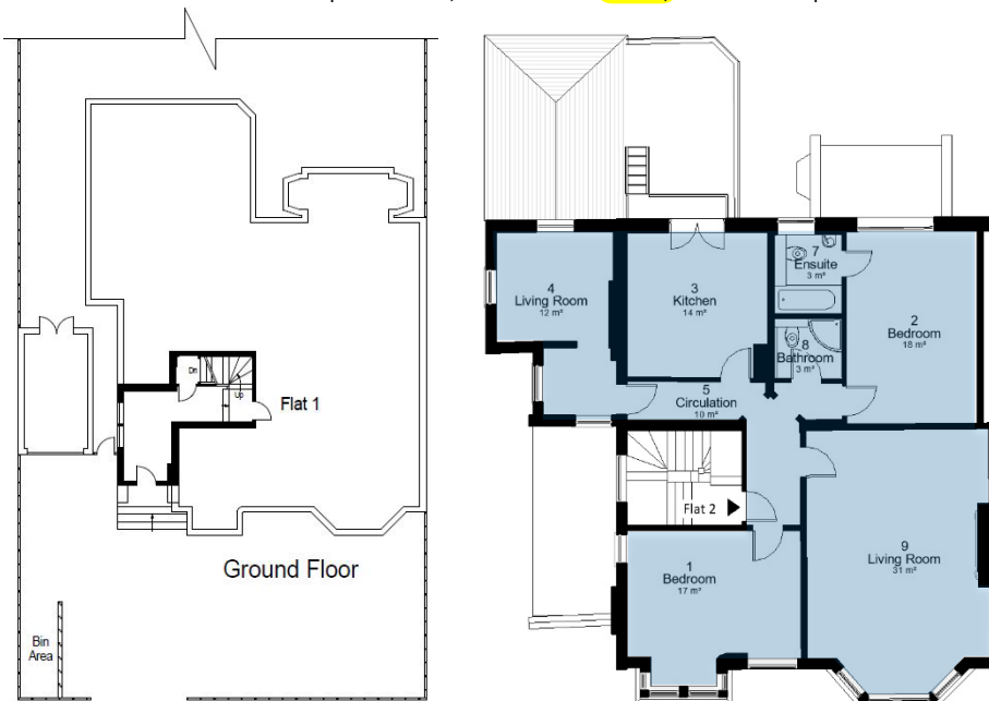
Existing Ground and First floor plans
