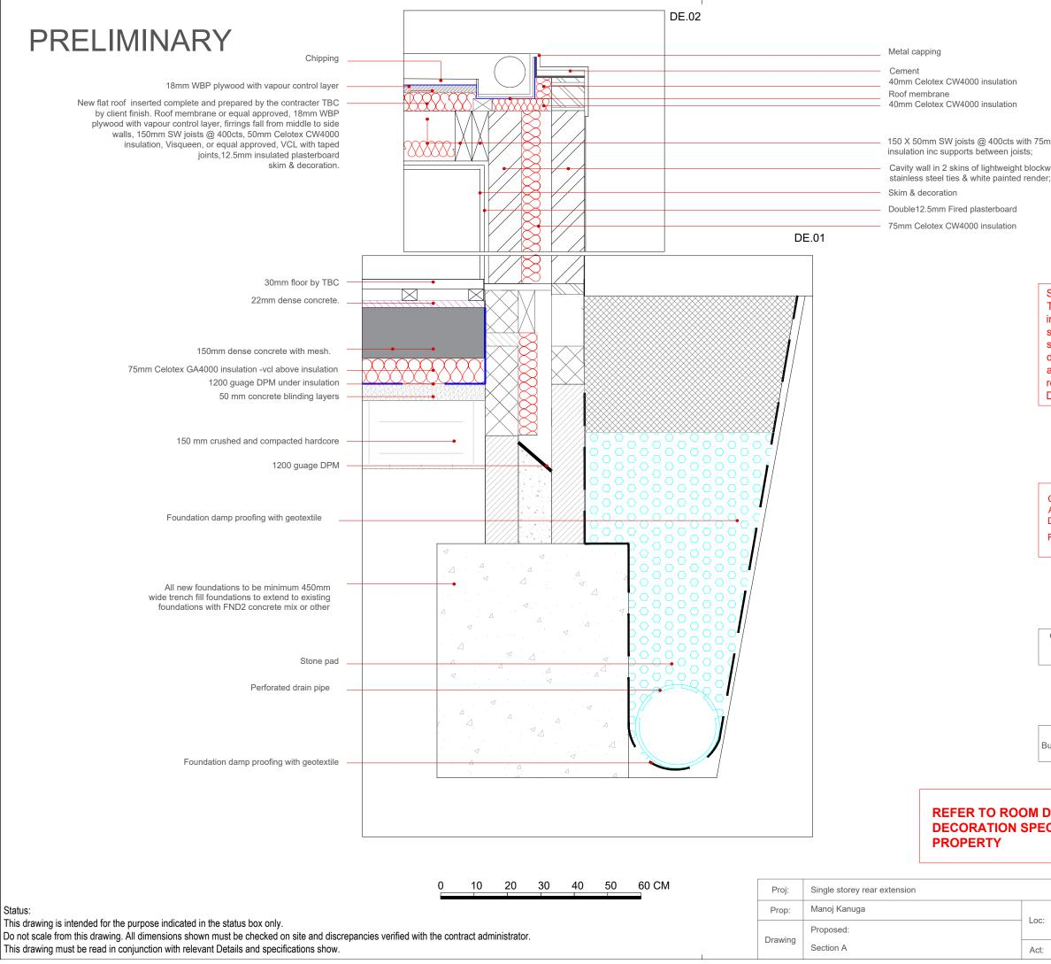
150 X 50mm SW joists @ 400cts with 75mm Xtratherm rigid
