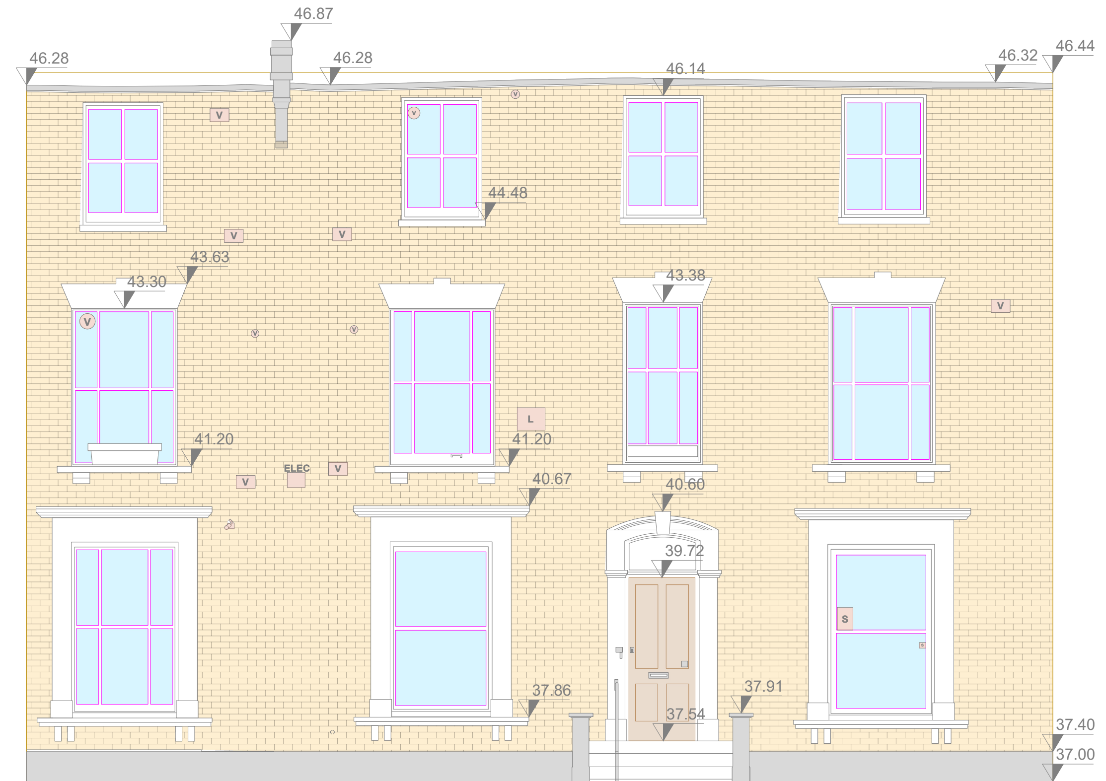
Existing South Elevation
