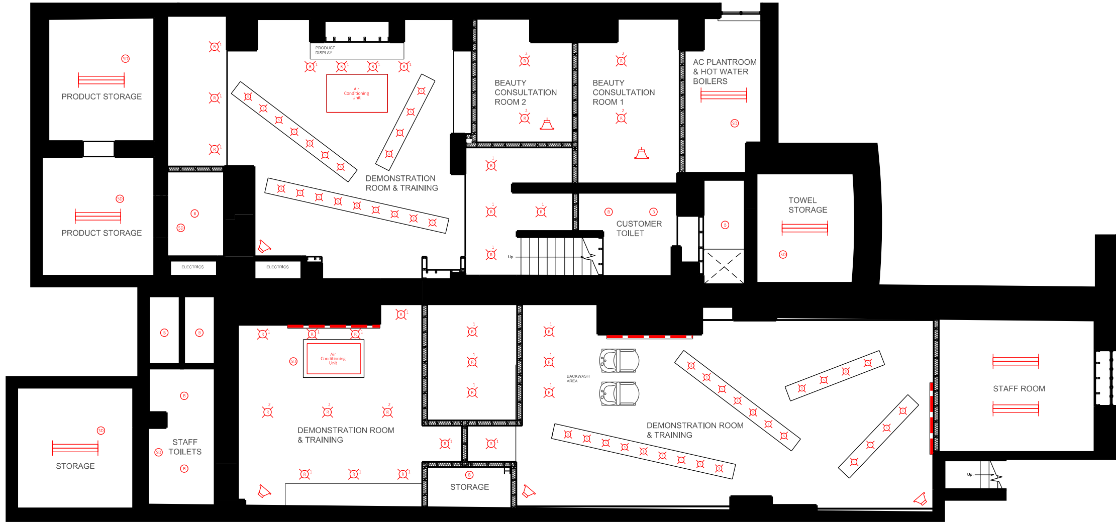
Existing Basement Floor Reflected Ceiling Plan
