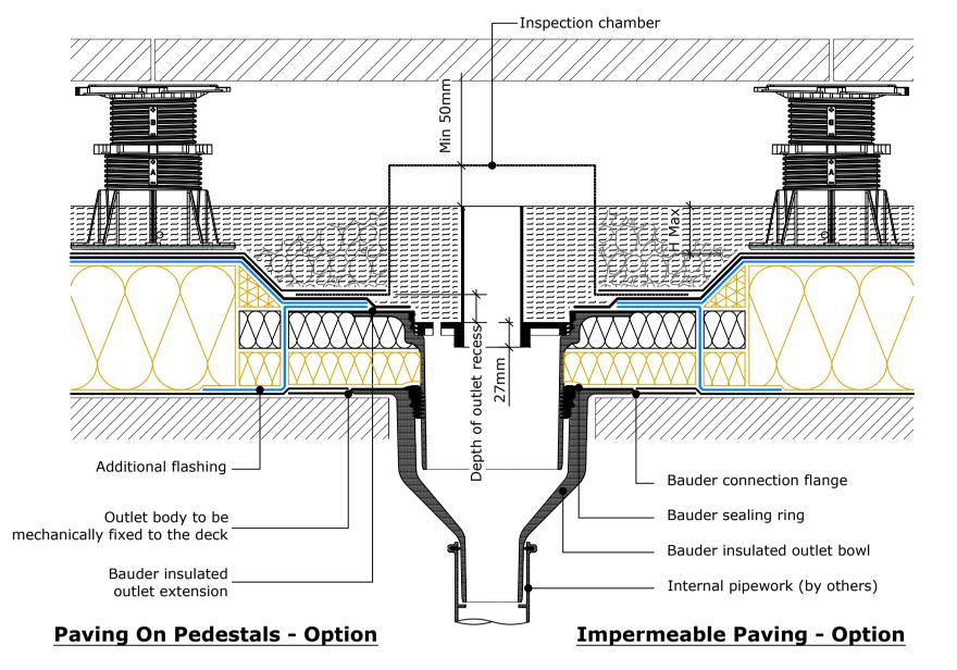
**Bauder Outlet - Bauder Bitumen Blue Roof Vertical Outlet DN70 - Sump** (Drg.No: D0000-00W\_BR\_006-Ext-SL-S-D4-AC\_002)
