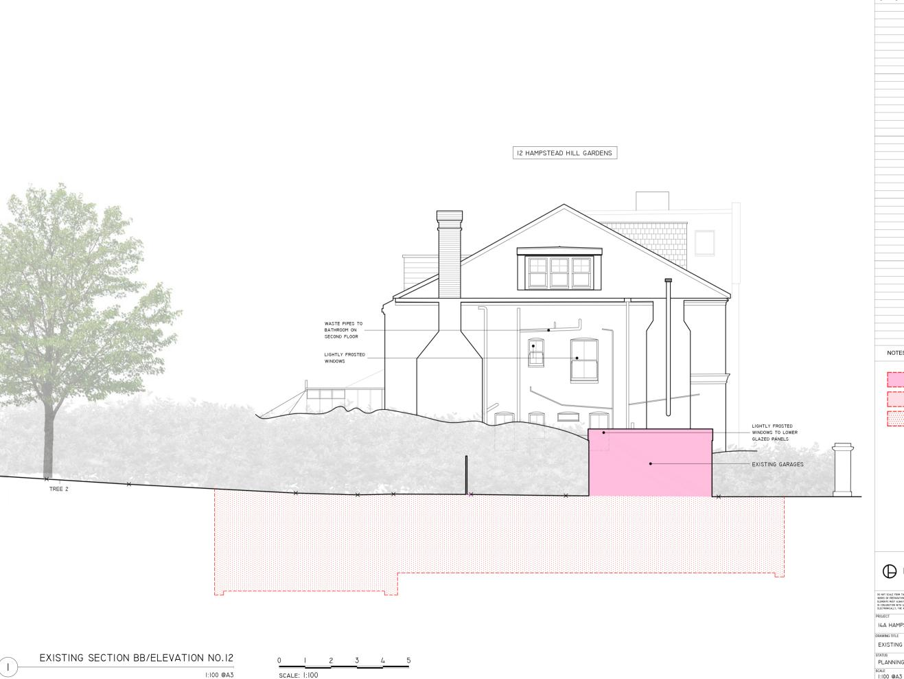
NOTES: PROPOSED DEMOLITION: EXISTING STRUCTURE PROPOSED DEMOLITION: EXISTING HARD LANDSCAPING PROPOSED EXCAVATION: EXISTING AREA TO BE REMOVED FOR BASEMENT
