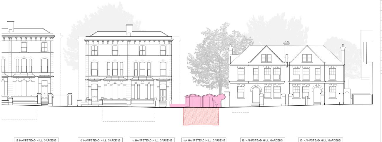
NOTES: PROPOSED DEMOLITION: EXISTING STRUCTURE PROPOSED DEMOLITION: EXISTING HARD LANDSCAPING PROPOSED EXCAVATION: EXISTING AREA TO BE REMOVED FOR BASEMENT
