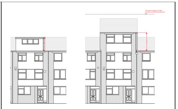
The proposal under consideration (below right) would be 2.9m at the roof eaves, an increase of 10cm above extant approval (below left) and 80cm increase above existing roof eaves. The height of the roof would be pitched to the roof ridge and would increase to 3.1m, an increase of 20.5cm above extant approval (also within the 3.5m limit of the GPDO).
