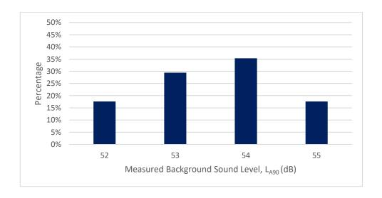
As shown in above histogram, our analysis has derived a noise emission limit of 54 dB  $L_{Aeq}$ , 1dB higher than the full daytime hours (07:00 – 23:00 hours) considered in the previously issued
