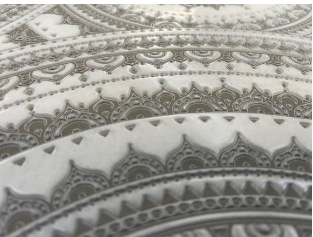
Fig. 2.3.2 Zoom in of polymer sheet cast from digital files
