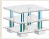
Strengthening existing columns and prop slab
